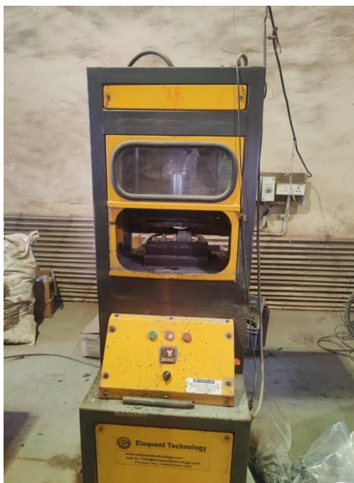
Photograph No. 14.1: Photograph showing core splitter used to split borehole cores
