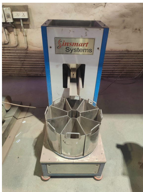
Photograph No. 12.3: Photograph showing coning-quartering equipment used in sample processing
