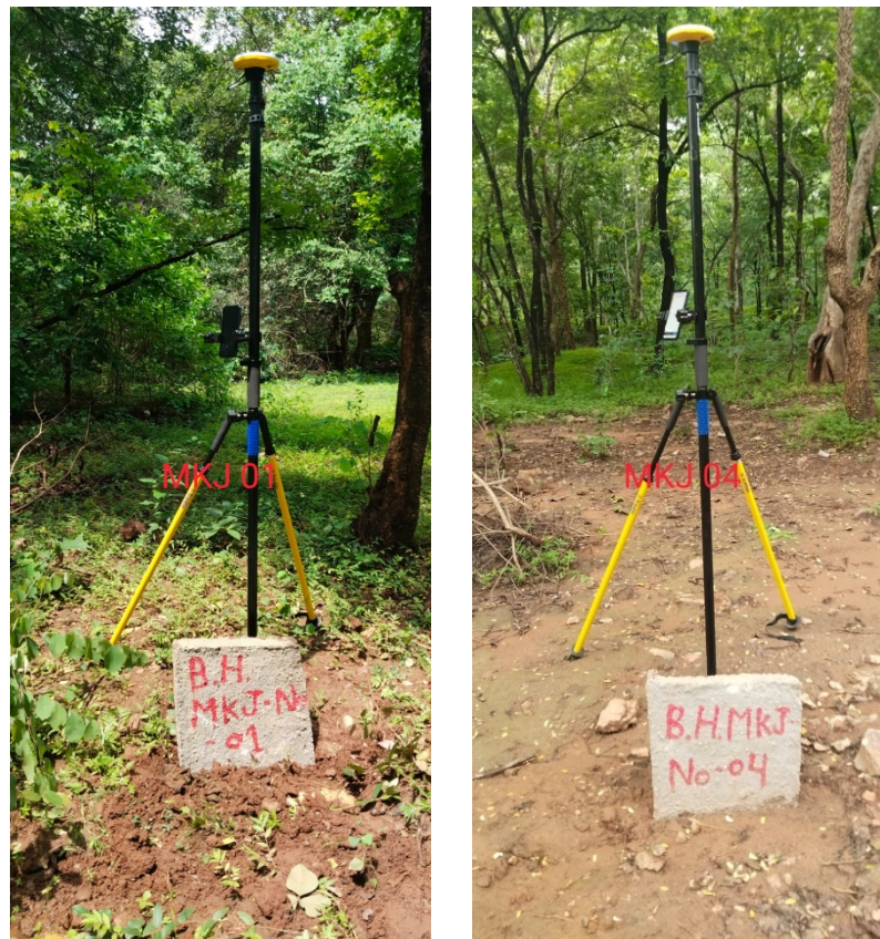
Photograph No. 11.1: Photograph showing high-precision DGPS measurement at the collar of Borehole MKJ-01 and MKJ-04 in the Katori Jhiriya Block
