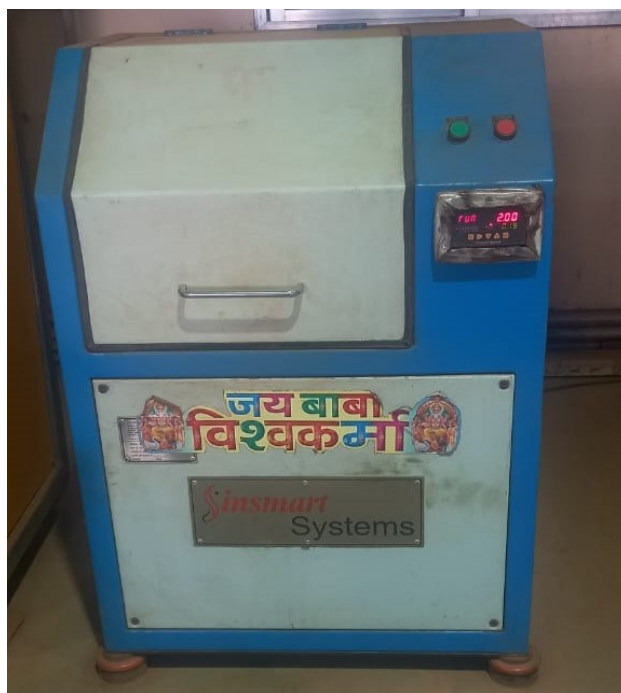
Photograph No. 12.2: Photograph showing pulveriser used in sample processing
