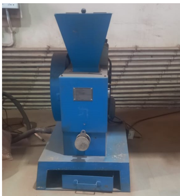
Photograph No. 12.1: Photograph showing sample sample crusher used in sample processing
